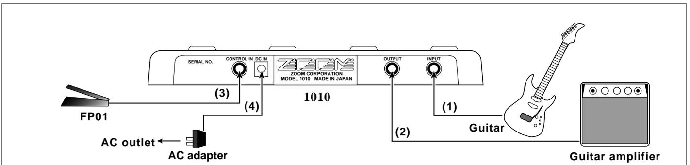
(1) Connect an electric guitar to the INPUT jack.
