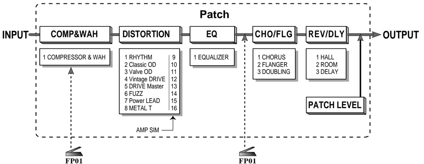
As shown in the illustration above, a patch of the 1010 contains parameters for the five types of effect modules and the patch level settings. In the Edit mode, you can call up any of these parameters and change them.
