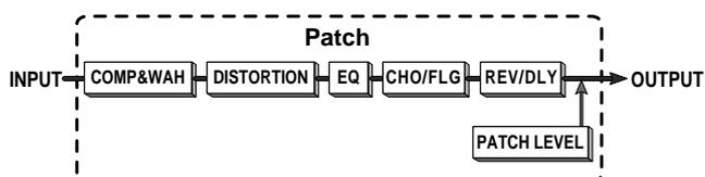
The 1010 has two memory areas or "groups" where patches are stored: the USER group for patches that can be altered and stored by the user, and the PRESET group for factory defined read-only patches. There are 12 patches in the USER group and 30 patches in the PRESET group, for a total of 42 patches.
