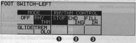
One of the three Rhythm Control functions can be selected. Pressing the footswitch executes the corresponding function:
