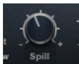
**SPILL** differentiates between vocal signal and unwanted ambient stage noise, to provide better tracking. (*Vocal Rider Live components only*)
