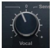
**VOCAL SENSITIVITY** controls the vocal detector sensitivity, which differentiates vocal content from noise floor, spill, and ambience, and identifies the beginnings and endings of words.
