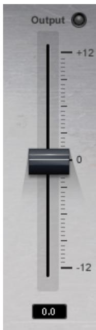
**OUTPUT** trims the vocal output gain, post-auto riding; the **CLIP LED** shows when output is clipping.
