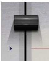
**RANGE MAX** sets the upper boundary of the Rider Fader movement range, setting the maximum Rider Fader gain.
