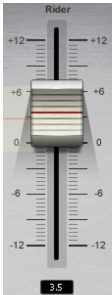
**RIDER FADER** is Vocal Rider's automatic control, which moves according to the internal detectors' algorithm to level-out the vocal, similar to manual fader riding. (The TARGET control is used to set the Rider Fader '0' calibration.)
