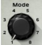
Mode sets the Front Profile Mode, determining which stereo content will remain in the L/R channels and which will feed the Center and Ls-Rs channels.
