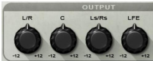
Output Trims provide up to 12dB boost or cut per surround stage: L/R, Center, Ls/Rs, and LFE.
