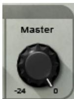
The Master Output Trim controls provides up to 24dB cut.
