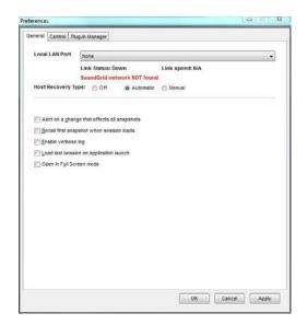
If you see the SoundGrid network NOT found message, and Local LAN Port is set to None, open the dropdown menu and set it to the LAN port connected to your SoundGrid network.
