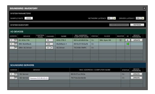
2. Hovering mouse over **IO: WSG-Y16** to view firmware version:
