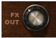
**FX OUT** controls the output level of the Effect path. (*Synth Type only*)
