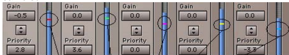
Relative Threshold markers. The relative threshold is adjusted by priority and bandwidth
