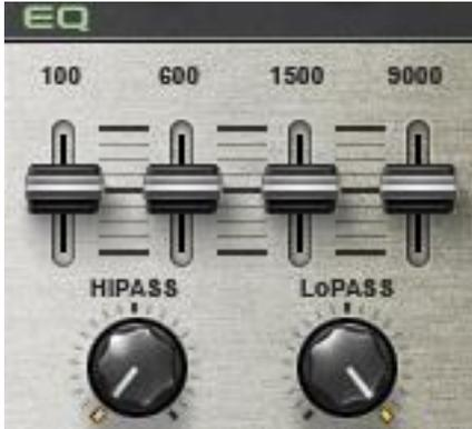
The EQ section is a 4-band fixed frequency graphic equalizer with high-pass and low-pass filters. At high boost levels, the EQ saturates with different tonal qualities than the Distortion module.
