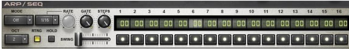
The ARP/SEQ section functions as both a traditional arpeggiator and a 16-step sequencer. Each sequencer step has an In/Out toggle as well as a pitch control which may be set +/-24 semitones from the currently held note.
