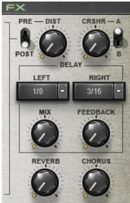
**DIST** controls the amount of distortion effect. Distortion is applied per voice, eliminating IMD (inter-modulation distortion.) Settings below 50% create a warm saturated drive effect; settings above 50% result in a more aggressive, “crunchier” sound.
