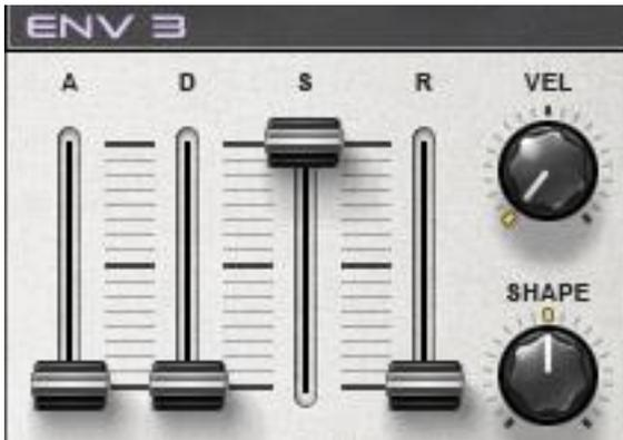
In addition to the filter and the VCA envelopes, Element 2.0 includes an envelope generator that can be freely assigned to selectable destinations via the modulation matrix.
