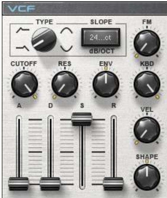
The VCF section includes selectable filter slope, frequency and resonance parameters as well as a filter envelope which determines the filter movement on each trigger.
