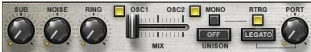
This section is used to combine OSC 1 and OSC 2, as well as add noise, sub-oscillation and ring modulation.
