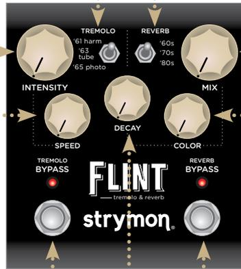
**MIX:** Controls the reverb wet mix from full dry at minimum to full wet with no dry signal at maximum. A 50/50 mix occurs around 3 o'clock on the mix knob.
