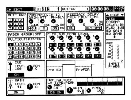
In this state, you can use the knobs and buttons of the VE-7000 to edit the following parameters.
