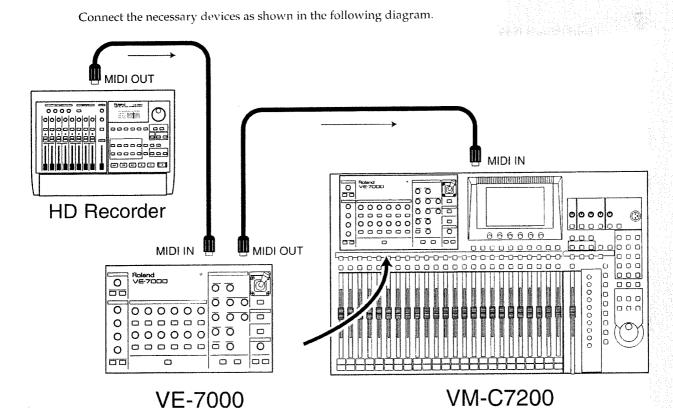
Use a MIDI cable to connect the VE-7000's MIDI OUT to the MIDI IN of the device (e.g., VM Console) that you wish to control from the VE-7000. If you wish to use the VE-7000 to control another device, such as an additional VM Console, connect the device to the MIDI IN of the VE-7000. MIDI messages that are input to the VE-7000's MIDI IN will be retransmitted without change from MIDI OUT, and sent to the MIDI IN of the VM Console or other device being controlled by the VE-7000.
