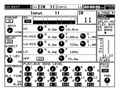
In this screen, the various knobs and buttons are in one-to-one correspondence with the operating panel of the VE-7000, making operation easy to understand.
