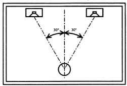
For best results the speaker should be placed close to the rear wall and far from the side wall. Do not place the speakers too far apart. Excessive room reverberation will also have an adverse affect upon the sonic result.
