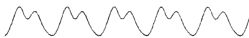
waveform of the decay portion 1.5 seconds after the attack of an electric piano
