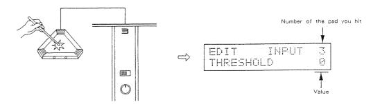
Step 4 Set the Threshold to an appropriate value by turning the Alpha Dial.
