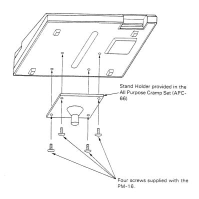
Install the PM-16 and Stand Holder onto the Pad Stand (MDS-1) as shown in the figure below.
