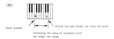
When a rhythm machine is used as the sound source, using the Dynamics Pitch, allows you to change the type of percussion sounds heard according to how forcibly the pad is hit.
