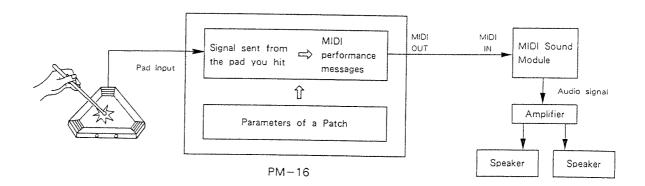
The combination of settings within the PM-16 that convert the signals sent from the pad as it is struck into MIDI messages, is called a patch. Up to 64 patches can be stored in the main unit's memory.
