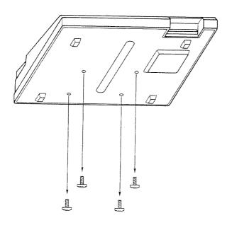
2Attach the Stand Holder from the All Purpose Clamp Set to the bottom of the PM-16 with the four screws removed in Step 1
