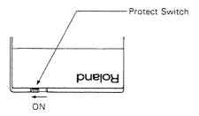
Step 2 Put an M-128D memory card into the main unit's Memory Card Slot as shown in the figure below.
