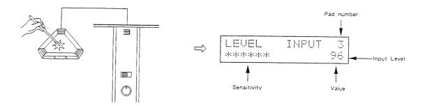
Step 5 Slowly turn the Sensitivity Knob clockwise, so that the strongest hitting of a pad will make the input level display between 110 and 125.
