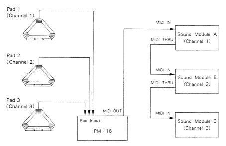
Hitting Pad 1 plays Sound Module A, Pad 2 plays Sound Module B. and Pad 3 plays Sound Module C.
