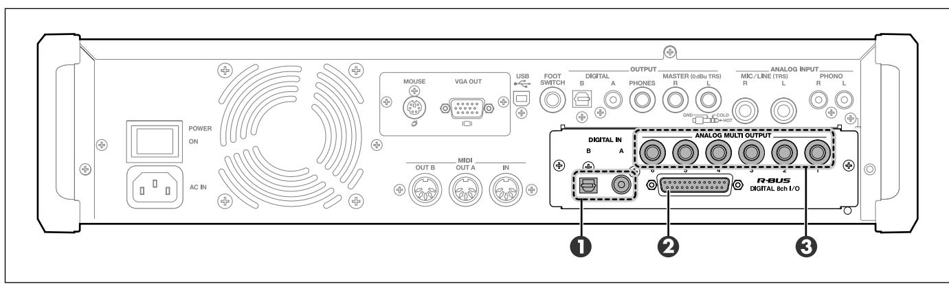
The illustration shows the MV-8800 rear panel when the separately sold MV8-OP1 option is installed.
