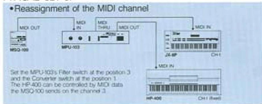
The MPU-103 MIDI Channel Filter/Converter reassigns the MIDI channel: It accepts MIDI data transmitted on the MIDI channel selected by the Filter switch, then sends that data on the MIDI channel selected by the Converter switch.
