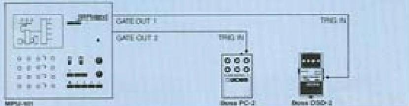
The MPU-101 converts MIDI data into analog signals. Connecting the MPU-101 to a MIDI sending unit, up to four conventional 1-volt/octave CV/gate synthesizers can be controlled by MIDI data.
