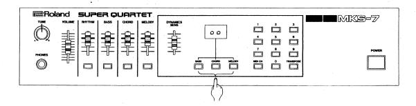
② Set the Dynamics Sens Knob to your taste. When the knob is moved even slightly, the previous setting will be deleted, and replaced with the current knob position.
