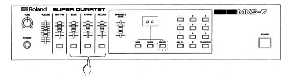
While the button is being pressed, the tone color currently called in that block will be heard in the pitch of A key.
