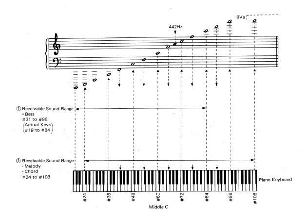
Above picture shows the sound range (7 octaves) of Note On/Off message that can be received by the MKS-7. If the data sent exceeds this range, it will be automatically transposed up or down to fit in the range.
