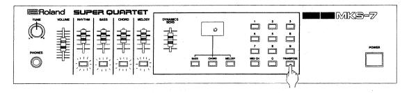
The Display **3** shows the number that represents how many semi-tones are currently transposed from the C key.
