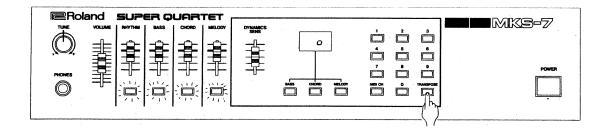
The Rhythm Button ①, Bass Button ②, Chord Button ③ and Melody Button ③ will all light up. These four buttons now serve as On/Off switches of the above 4 MIDI messages as shown right. When the button is lighted, the corresponding message will be received.
