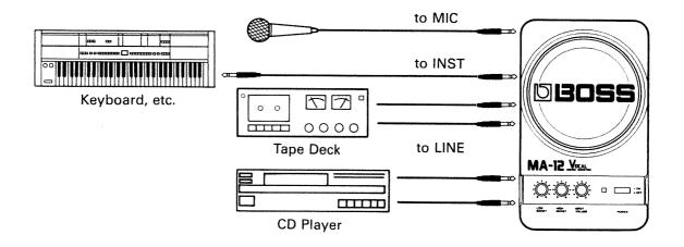
\* Inputs, INST and LINE, can be used at the same time. Input the signals of Lch and Rch to the INST and the LINE respectively when playing a stereo source in monaural. The devices to be connected to Inputs INST or LINE cannot be connected to the Input MIC.
