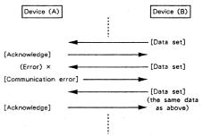
Device (B) rejects the data re-transmitted, and completes data transfer.
