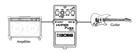
These settings produce a really powerful distortion. The unit should be connected so it is located before a distortion-type effects unit.
