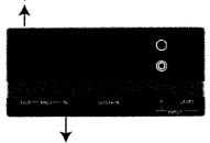
To the MIDI OUT connector of the other instrument (or the "IN" connector of the supplied MIDI/Joystick cable)
