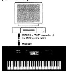
Note: If you also connect the EM-50/30's MIDI IN port to the sequencer's MIDI OUT port, be sure to switch of the sequencer's Soft Thru (or MIDI Echo) function. See its manual for details.
