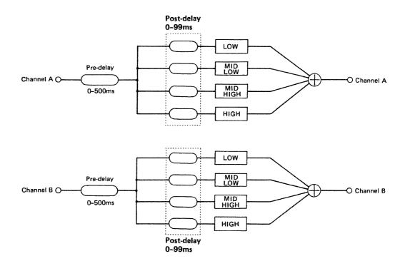
In this mode, the E-660 works as a 2 channel, 4 band, band-pass filter, allowing you to set parameters separately for each channel. The Pre-delay (maximum 500ms) and Post-delay (maximum 99ms) can be set individually for each channel.
