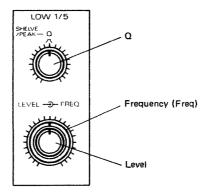
Q.....This curve controls the width of the frequency band. Freq....This sets the center frequency where the level is changed.
