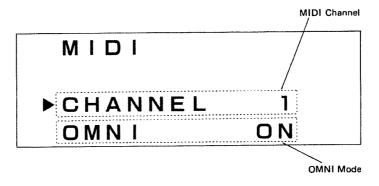
PROCEDURE 2 To set the MIDI channel, move the ▶ mark to the "CHANNEL" position with the Select Button. To set the OMNI Mode, move the ▶ mark to "OMNI".
