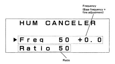
PROCEDURE 5 Using the Select Button, move the ▶ mark to the "Freq" position.
