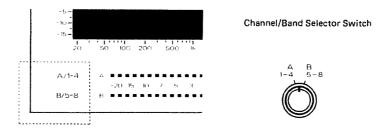
\*When the parameter setting display (=after the EQ Button is pressed) or the graphic display is shown, the A/1-4 or B/5-8 Indicator changes according to the position of the Channel/Band Selector Switch. However, in any other display, the indication does not correspond to the switch position. To correct this, simply change the positions of the switch until they come to match.
