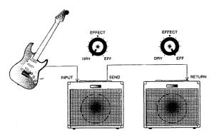
O If you want volume control after distortion is applied in the preamp stage, just connect a volume pedal (optionally available; BOSS FV-300L, FV-50L) in the loop.
