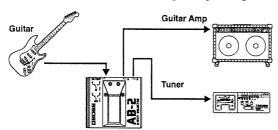
Connecting as shown here allows you to mute the sound from the guitar amp when tuning the instrument.
