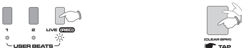
Activate the FILTER/LFO effect, check the MASTER is set to ON and that the FX MIXER joystick is pointing towards the effect or in the central upright position. Now, use the 'TAP' button to trigger the FILTER effect in time with a particular part within the music, perhaps the bass line.
