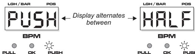
Further fine adjustments can be made beyond the 'PUSH ½ beat' point (display reads from '+13' up to '+23') until the synchronisation is pushed forwards by one complete beat (maximum PUSH adjustment). For this setting the display will show the following:
