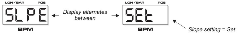
When the 'SET' slope is selected, the rise/fall time will always be equal to the quantize setting e.g. if the quantize is set to 16's, the slope duration will be fixed at 1/16 of the beat. This gives a very short, punchy feel to the trigger pattern.
