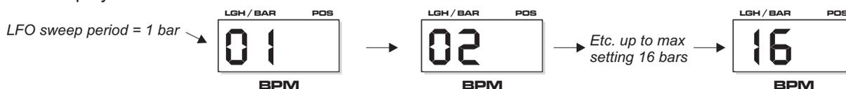
RANGE = 01, 02, 03, 04, 08, 12, 16 BARS. The LFO can be re-started from the beginning of the wave shape each time the MASTER or filter ACTIVATE button is pressed.
