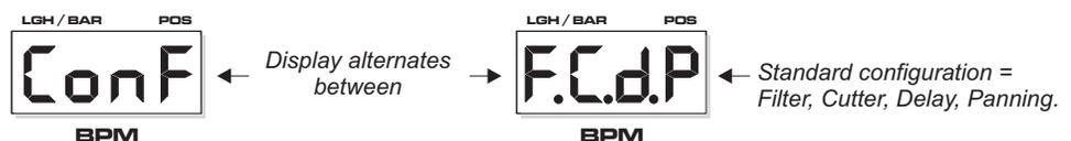
The effects can be arranged one after the other in any order you wish. Try various combinations to hear the way the interaction between the effects changes. To change the configuration, use the effect 'ACTIVATE' buttons to select the effects in the order you want to place them.
