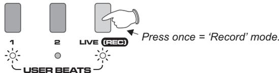
In 'Record' mode, the selected Memory / LIVE(REC) indicators will change to 'on'. The FEDERATION gives you a 4 beat count-in (with audible 'beep' if required) before recording starts. The 'POS' (beat position) digit in the main BPM display will stop flashing '1' and change to show the count-in, as in the following example:
