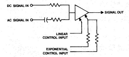
DC SIGNAL IN - This is a direct coupled input to the VCA. A DC voltage applied to this input will appear as an inverted DC level at the output. The output level is controlled by both the linear and exponential control inputs.
