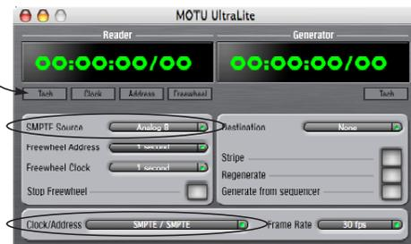
Launch the MOTU SMPTE Setup software to specify the time code input, frame rate and amount of freewheel. Also, confirm that the *Clock Source/Address* is *SMPTE/SMPTE*.
