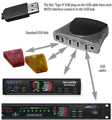
Figure-5: An inexpensive, standard USB hub, such as the mac hub4U™ shown above from Entrega, allows you to connect multiple MOTU USB MIDI interfaces. You can even mix and match different models of MOTU interfaces, using the combination that best suits your needs for synchronization, number of MIDI ports, etc.
