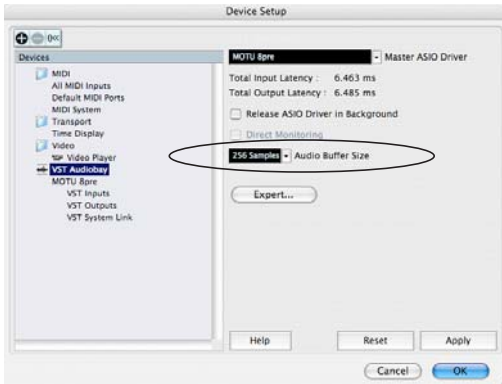
Figure 10-4: In Cubase SX or Nuendo, choose Devices menu > Device Setup and click VST AudioBay to access the window above and the Audio Buffer Size setting.
