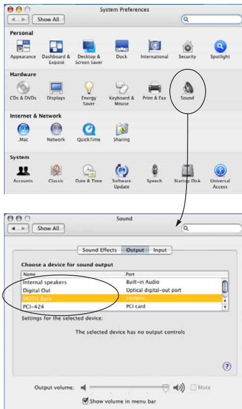
Figure 5-2: The Mac OS X sound preferences let you use the 8pre for general stereo audio input and output for your Mac.
