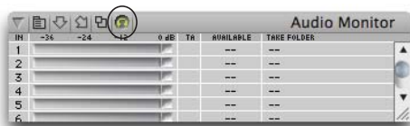
Figure 10-7: Enabling CueMix DSP in AudioDesk or Digital Performer. Note: the 'Only during recording...' and 'Always' options are for AudioDesk 2 and DP4 only. DP5 has expanded input monitoring features. Consult your DP5 documentation.
