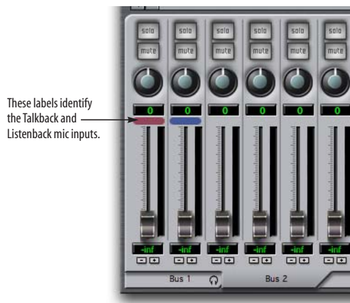
Figure 11-4: The purple label identifies the Talkback mic input; the blue label indicates the Listenback mic. Use the input fader to control the mic volume.
