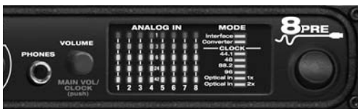
Figure 6-1: The VOLUME knob is a push-button rotary encoder.
