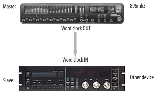
Figure 4-17: Slaving another digital audio device to the 896mk3 via word clock. For the 896mk3 clock source, choose any source besides word clock, as it is not advisable to chain word clock.
