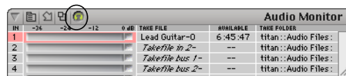
Figure 6-3: To enable the CueMix™ Plus Auto Monitor feature in AudioDesk or Digital Performer, be sure the ‘Direct hardware playthrough’ option is chosen, and be sure audio patch thru is turned on.
