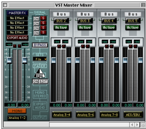
Figure 8-4: Use the output buttons at the bottom of each channel strip to assign MOTU 896 outputs to busses. You can then assign channels in the Monitor window to each bus as desired.
