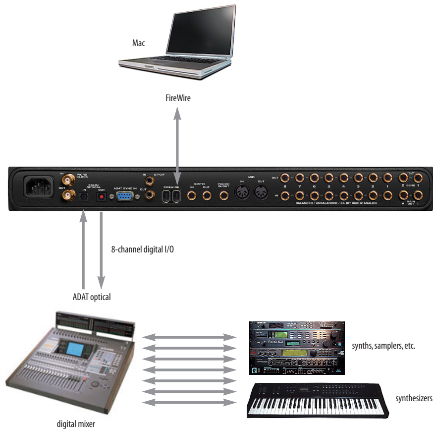
Figure 3-6: Using the 828mkII with a digital mixer.
