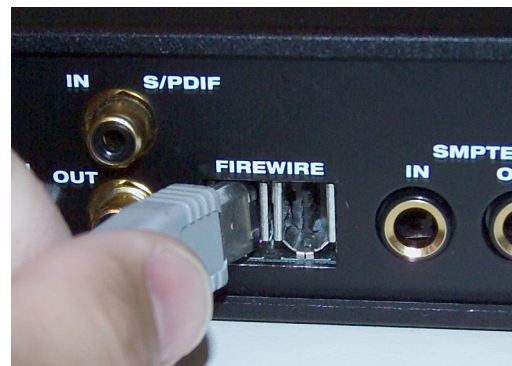
Figure 3-1: Connecting the 828mkII to the computer.
