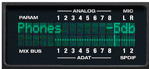
Figure 7-3: For many settings, the LCD “zooms in” on the setting as you adjust it.
