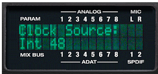
Figure 7-2: In setup mode, the LCD displays a setup parameter in the top row of the LCD and the current setting in the bottom row.
