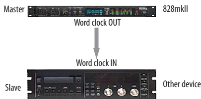
Figure 3-18: Slaving another digital audio device to the 828mkII via word clock. For the 828mkII clock source, choose any source besides word clock, as it is not advisable to chain word clock.
