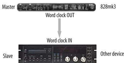
Figure 4-19: Slaving another digital audio device to the 828mk3 via word clock. For the 828mk3 clock source, choose any source besides word clock, as it is not advisable to chain word clock.
