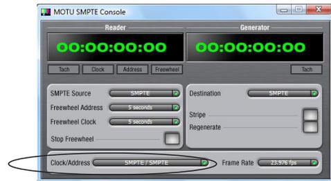
Launch the MOTU SMPTE Console and specify the *SMPTE Source*, which is the interface receiving the SMPTE time code. Also, confirm that the *Clock Source/Address* is *SMPTE/SMPTE*. For details about the other settings, see chapter 12, "MOTU SMPTE Console" (page 99).
