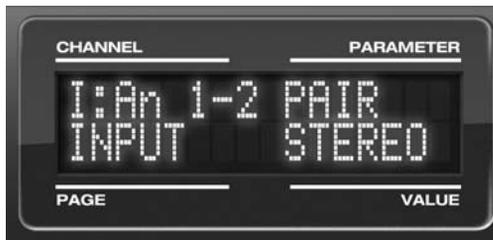
Figure 4-6: The settings for analog inputs 1 and 2 (as a pair).
