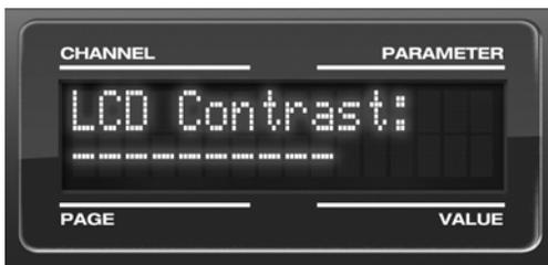
Figure 6-5: In setup mode, the LCD displays a setup parameter in the top row of the LCD and the current setting in the bottom row.
