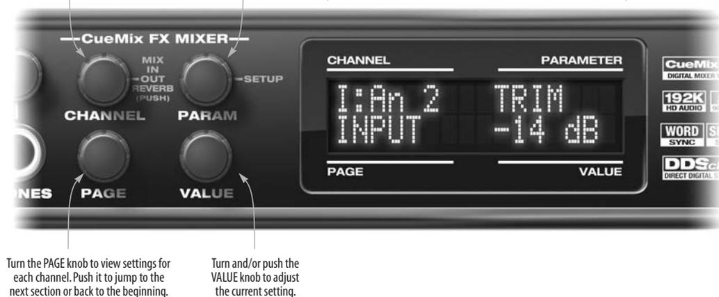
Figure 6-3: The 828mk3 front panel controls.
