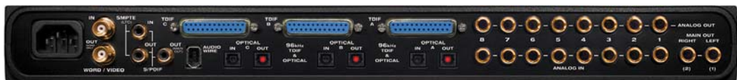
Figure 4-2: You can connect up to three ADAT optical devices, three Tascam TDIF devices, eight analog and two SPDIF devices to the 2408mk3.
