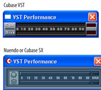
Figure 7-9: Keep the Audio Performance window open to keep tabs on your computer’s processing power and hard disk performance.
