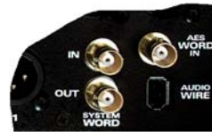
Figure 4-14: Resolving the AES/EBU output to its own independent word clock.
