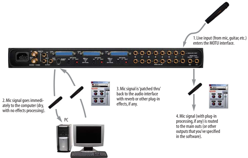
Figure 10-1: There are two ways to monitor live audio inputs with a PCI-424 system: 1) through the computer or 2) via CueMix™ DSP hardware monitoring. This diagram shows method 1 (through the computer). When using this method, use the PCI-424's 'Samples Per Buffer' setting to reduce the slight delay you hear when monitoring the live input, but don't lower it too much, or your computer will act sluggish.
