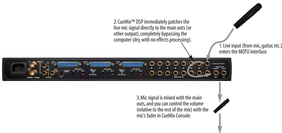
Figure 10-2: This diagram shows the signal flow when using CueMix™ DSP no-latency monitoring. Notice that this method does not allow you to process the live input with plug-ins in your audio software while it is being monitored. You can, however, add effects later — after recording the live input as a disk track. CueMix™ DSP lets you hear what you are recording with no delay and no computer-based effects.
