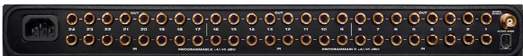
Figure 4-6: You can connect up to 24 analog inputs and outputs to the 24I/O.
