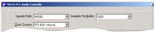
Figure 6-1: The PCI-424 settings at the top of the window are global settings that apply to the system as a whole, regardless of the MOTU PCI audio interface connected to it.
