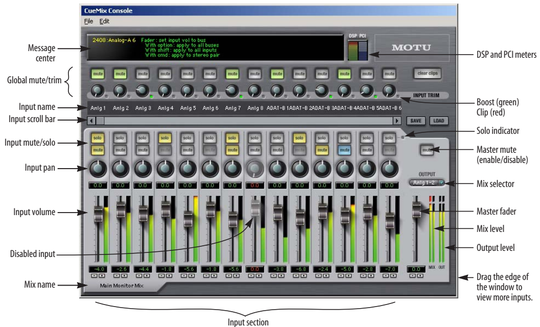
Figure 11-1: CueMix Console is a virtual mixer that gives you control over the PCI-424 card's on-board mixing features.
