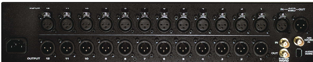
Figure 4-7: You can connect up to 12 analog inputs and outputs, plus stereo AES/EBU, to the HD192.
