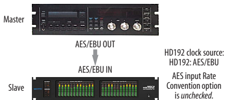
Figure 4-10: Slaving the HD192 to an AES/EBU device. For the HD192's clock source, choose 'HD192: AES/EBU'.
