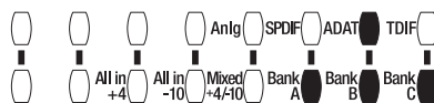
Figure 5-9: Choosing a source for a transfer. Press the SET button repeatedly to choose Bank A, B or C, or all three combined as shown.
