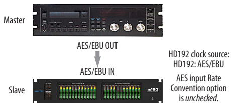
Figure 3-10: Slaving the HD192 to an AES/EBU device. For the HD192's clock source, choose 'HD192: AES/EBU'.
