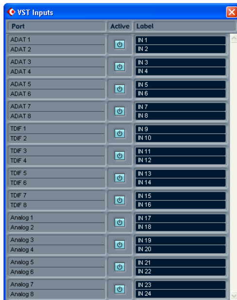
Figure 9-5: Activating PCI-424 inputs in Nuendo.
