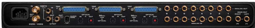
Figure 3-2: You can connect up to three ADAT optical devices, three Tascam TDIF devices, eight analog and two SPDIF devices to the 2408mk3.
