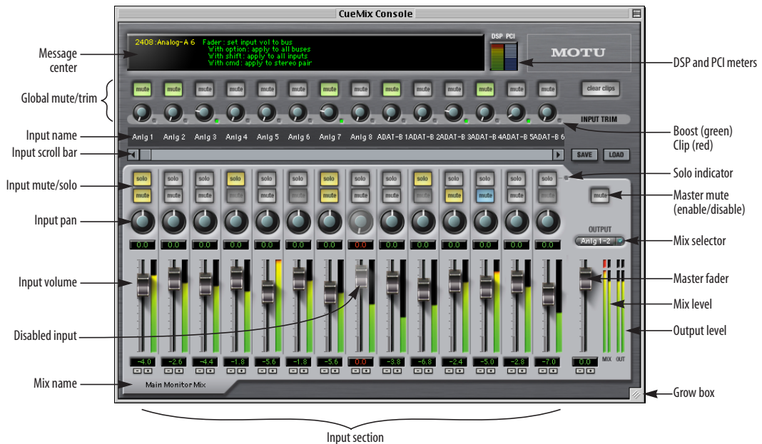
Figure 13-1: CueMix Console is a virtual mixer that gives you control over the PCI-424 card's on-board mixing features.
