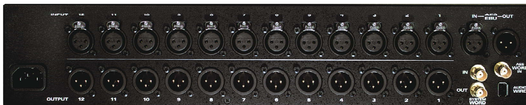
Figure 3-7: You can connect up to 12 analog inputs and outputs, plus stereo AES/EBU, to the HD192.
