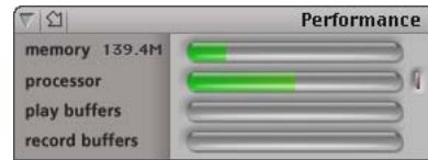
Figure 7-4: Keep the Audio Performance window open to keep tabs on your computer’s processing power and hard disk performance.
