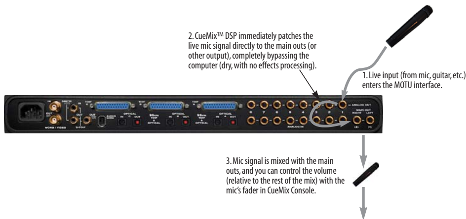
Figure 12-2: This diagram shows the signal flow when using CueMix™ DSP no-latency monitoring. Notice that this method does not allow you to process the live input with plug-ins in your audio software while it is being monitored. You can, however, add effects later — after recording the live input as a disk track. CueMix™ DSP lets you hear what you are recording with no delay and no computer-based effects.
