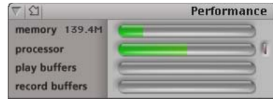
Figure 7-2: When adjusting the ‘Samples Per Buffer’ to reduce patch thru latency, watch the ‘processor’ meter in the Performance Monitor. From the Windows menu, choose Performance Monitor. If you hear distortion, or if the Performance meter is peaking, open CueMix Console and look at its message center for hints as to what’s going on.
