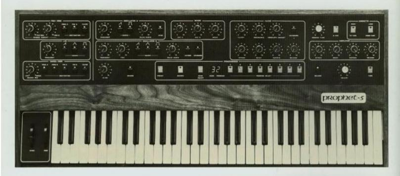
The **PROPHET** 5 from Sequential Circuits is a completely programmable polyphonic synthesizer, the world's first in fact. The **PROPHET** has 5 complete voices with two voltage controlled oscillators, a noise source, a voltage controlled lowpass filter and two 4 stage envelope generators per voice. The voices can be controlled by either the front panel knobs and switches or by one of the programs in storage.
