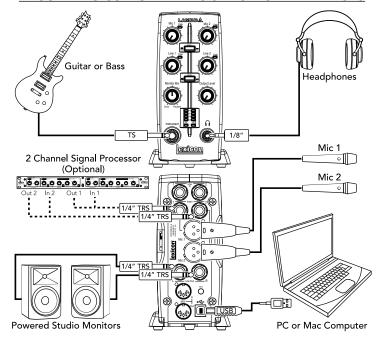
NOTE: When connecting to the Instrument input, the LINE 1 input will be deactivated.
