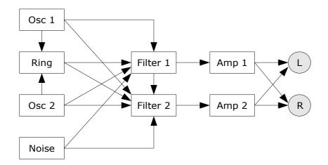
Each voice of the *blooo* features two oscillators feeding a Ring modulator. The individual outputs of the oscillators, the Ring modulator, and an additional white noise generator are sent to the input mixers of two multi-mode filters; furthermore, Filter 2 can receive the output of Filter 1. The filter outputs are routed to two individual amplifiers with panorama control which are connected to the main stereo output bus.
