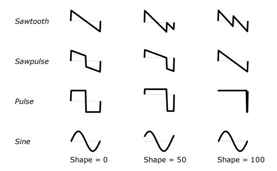
Note that *Sawtooth* with a shape value of 100 equals a mixture of a sawtooth wave and an additional sawtooth wave transposed by one octave. For *Sine* the shape value controls the phase of the sine waveform only.
