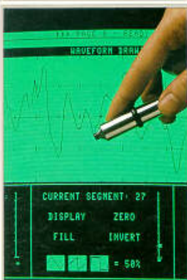
The Lightpen can be used directly to draw waveforms or alter those already in the memory.
