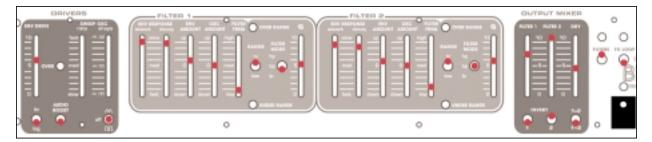
**Highpass Dual Down Drive:** Chunky sweep, which is good for heavily accented lines and adds percussiveness to your attack. Try out different settings of the Filter RANGE, MODE, INVERT, and MIX controls.
