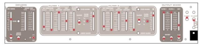
**Sci-Fi Sweep:** The LFO is acting on the Filters with a falling sawtooth waveform. In the Output Mixer section, the filters are set to sound like a Phasor when swept.
