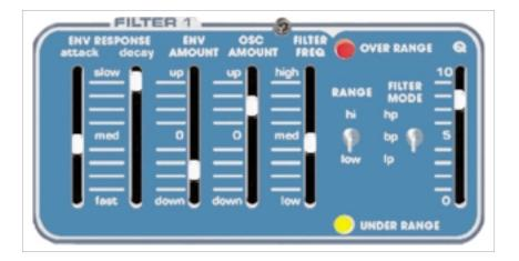
**NOTE**: FILTER 1 and FILTER 2 HAVE IDENTICAL CONTROLS AND RESPONSE, BUT ARE SEPARATELY ADJUSTABLE.
