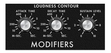
The Loudness Contour section is an ADS envelope generator/VCA combo used to dynamically shape note volume. If you're not familiar with the operation of ADS envelope generators, here's an overview:
