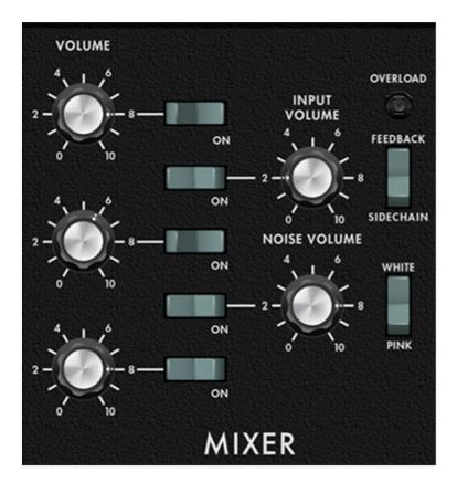
Mixes the signal levels of all three oscillators as well as Miniverse's noise source and "external" sidechain or feedback signal.
