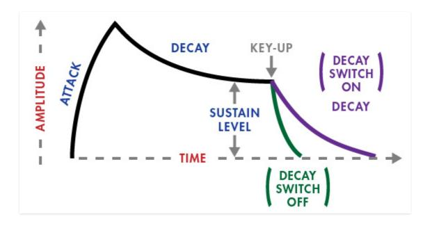
When Miniverse receives a gate voltage from a keyboard note being played, the contour generator outputs a dynamically changing voltage, according to the settings of its stages. The Attack Time stage defines how long it takes for the output voltage to rise from 0 to 5 volts.
