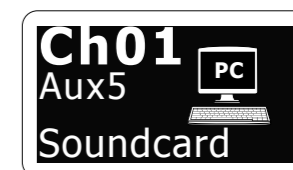
Example: Channel 01 has the nickname Soundcard and is fed from Aux input 5.
