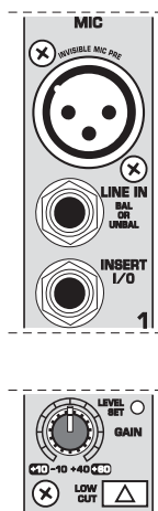
Fig. 2.1: Connectors and controls of mic/line inputs
