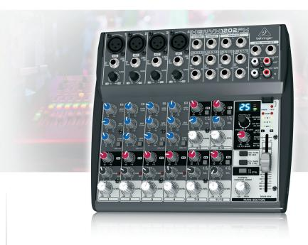
The compact XENYX 1202FX mixer allows you to effortlessly achieve premium-quality sound, thanks to its 4 onboard studio-grade XENYX Mic Preamps and ultra-musical "British" channel EQs. Add to this our 24-Bit, dual engine FX processor with 100 awesome presets including reverb, chorus, flanger, delay, pitch shifter and various multi-effects – and the 1202FX becomes an incredibly versatile mixer for your live performances.
