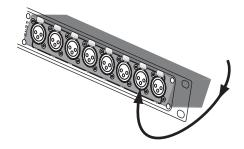
4. Attach the module to the patch panel. Each PB28 Series module comes with 16 screws that are used to secure it to the front of the PB28 Patch Panel. Always install all 16 screws.
