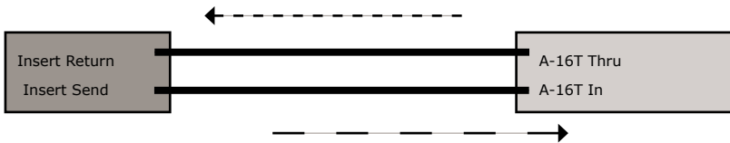
Separate cables connect signals into the A-16T and back into the console
