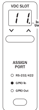
VDC Slot 11 on the 6416dio is set to receive GPIO In from the rear-panel jack.
