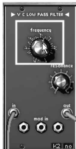
The setting of filter1 cut-off frequency
