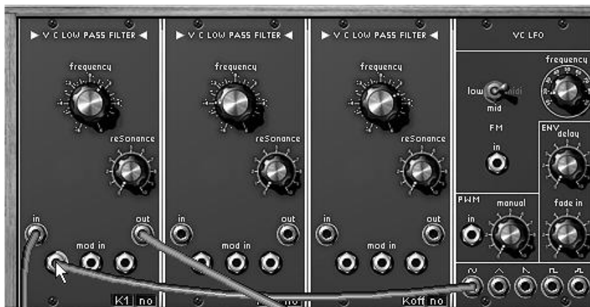
Connection of LFO to filter1
