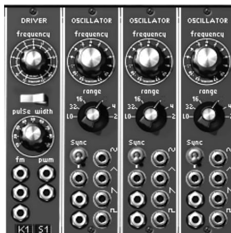
An oscillator bank: 1 "driver" and 3 "slave oscillators"
