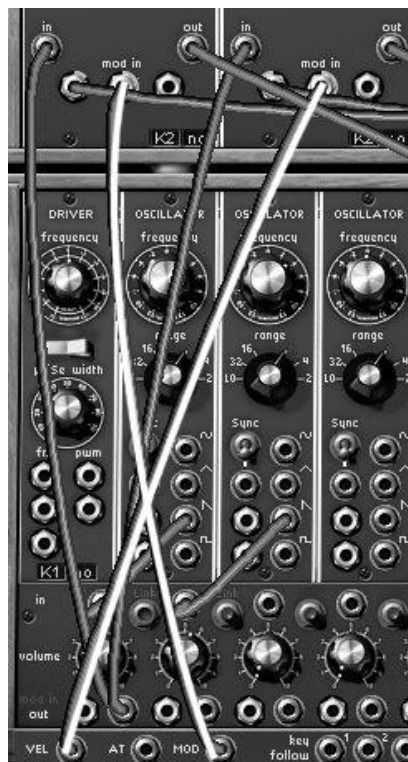
Connections for modulation and velocity outputs on the frequency modulation of filters 1 and 2
