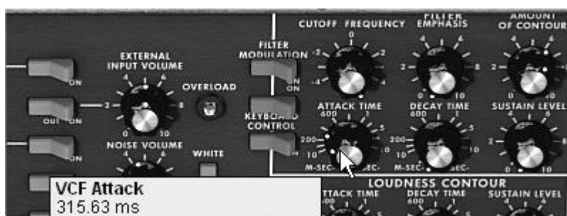
The "Attack time" parameter of the filter envelope
