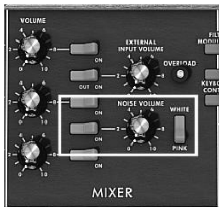
The noise generator set on the mixer
