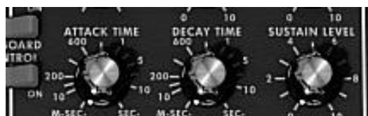
Envelope generator associated to the filter
