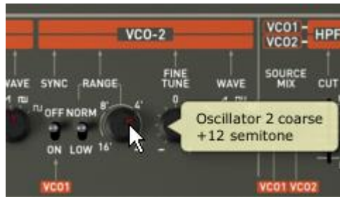
Tuning the second oscillator
